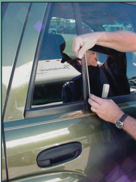
6. Lever the linkage rod forward to unlock the door.
